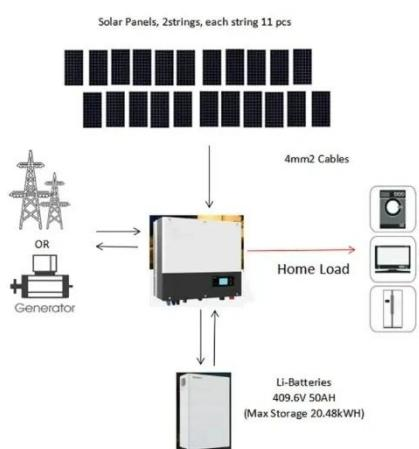
Li Battery \* 3 6 input, 2 output control box \* 2 MPPT Controller \* 2 ...
