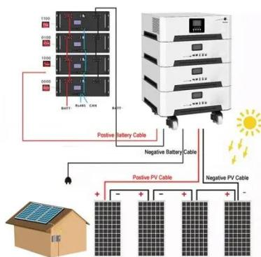
system This scheme is applicable to the distribution system composed of, energy storage, power load and power grid (generator). The ...
