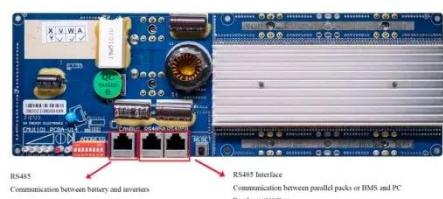
RS485 Communication between battery and inverters Baud rate 9600bps
