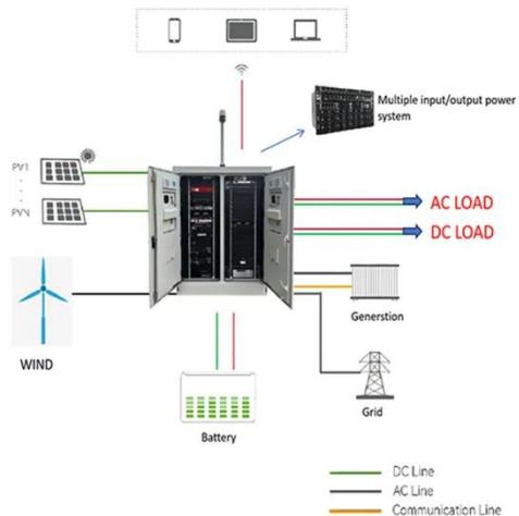
power generation equipment Base station energy cabinet: a highly integrated and intelligent hybrid power system that combines multi-input ...
