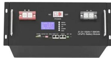
51.2V 150AH, 7.68KWH
